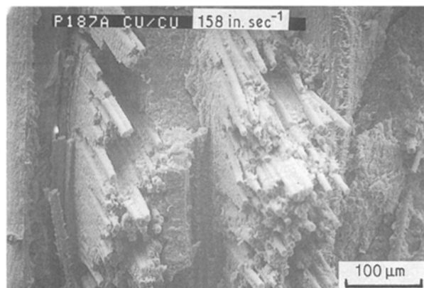
Figure 17 Scanning-electron photomicrographs of the failure surfaces for the double-sided copper laminate.
